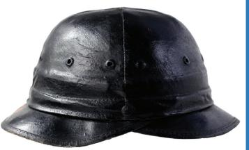
in shellac for durability, and fitted the inside with a suspension device to distribute the force of an impact. Dubbed the Hard Boiled Hat due to the steaming process, Bullard's creation was patented in 1919 and became the world's first commercially-available head protection gear.
